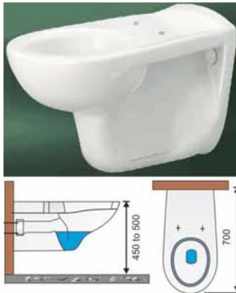
Figure 9.2d: Mounting Height of EWC
