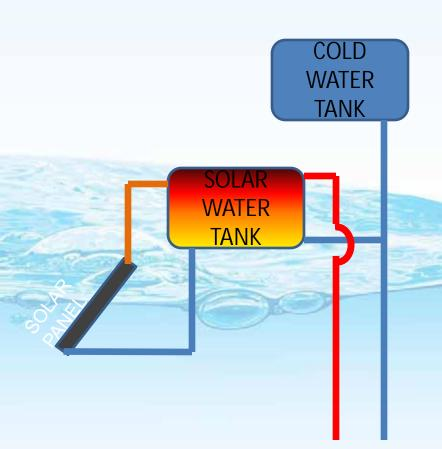
. Hot water being lighter than cold water, rises to the top of the collector and into the hot water tank.
