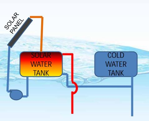
Cold water from the cold water tank is forced into the battery of collectors.
