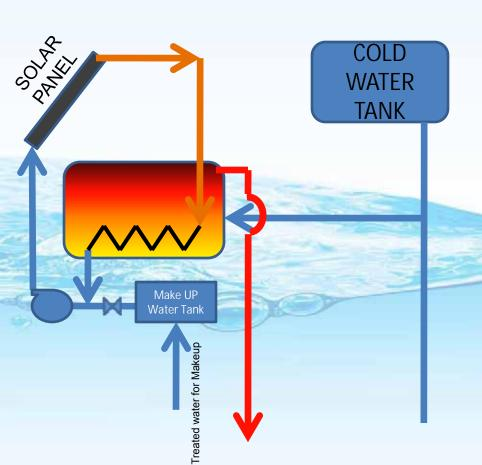
In case if water quality is not good, this system can be installed.
