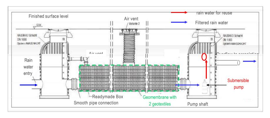
The rain water may be collected and storaged in a readymade basin/ storm cell storage completely sealed using a geomembrane such as HDPE. The extraction of water is done in pump shaft outside the basin. A filter is use before introduction of the rain water in the basin.
