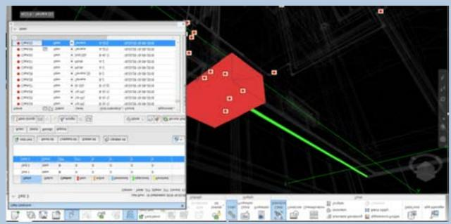
*Fig 10A: Pipe clash with duct*
