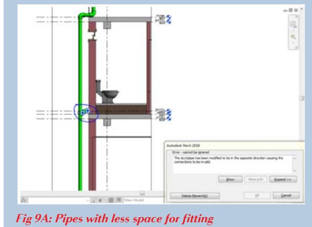
*Fig 9A: Pipes with less space for fitting*
