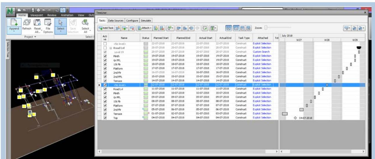
*Fig 11: Work schedule of plumbing work (installation)*
