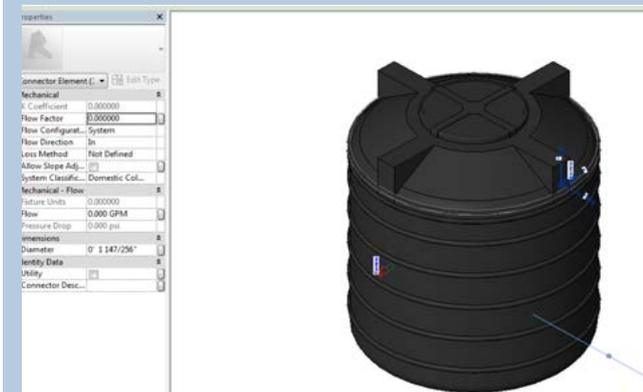
*Fig 8: Water tank with properties*
