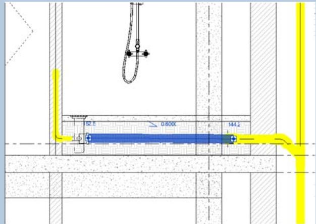
**Fig 4: Waste Water pipe with slope 1:60**
