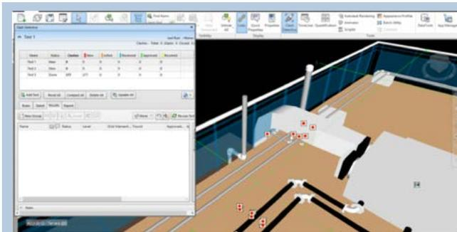
*Fig 10: Pipe clash with duct*
