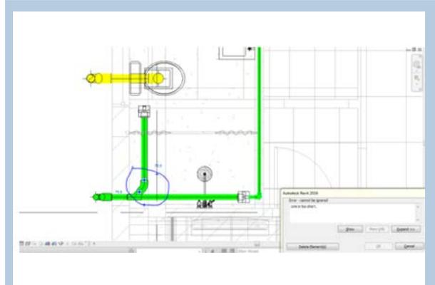
*Fig 9: Pipes with less space for fitting*
