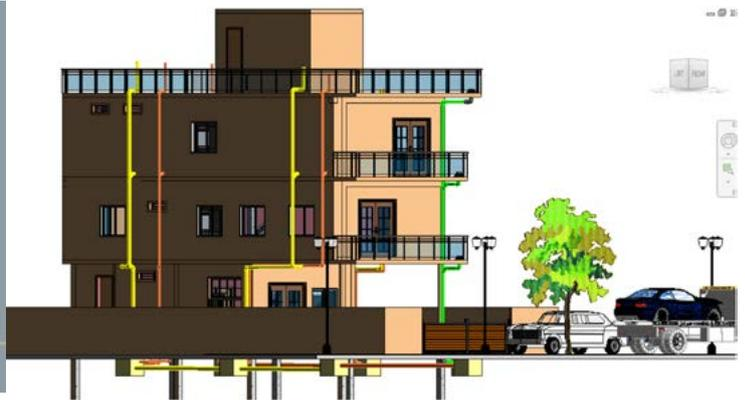
Fig 2: 3D model with sanitary pipes outside
