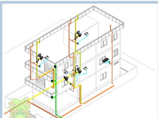
**Fig 6: 3D model with different color sanitary pipes**
