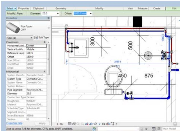
**Fig 3: Water supply lines with properties of pipe**
