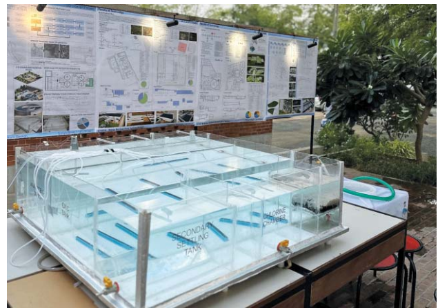
1:1 Scale A2O Based Conceptual Packaged Sewage Treatment Plant Model
