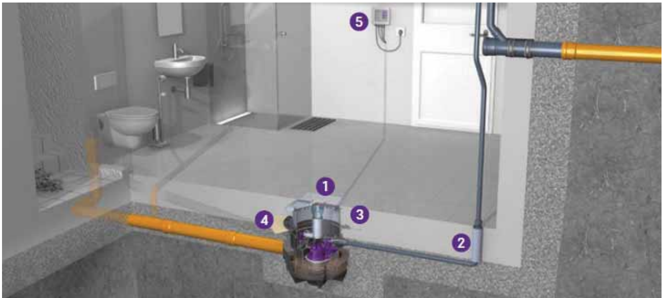
1 Lifting station 2 Pressure pipe set 3 Extension section 4 Gasket set 5 Control unit
