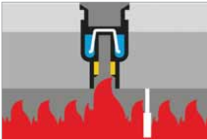
Pipe loosens due to extreme heat exposure
