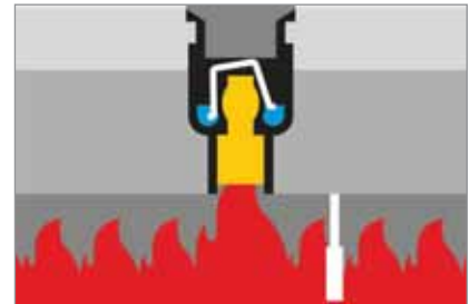
Drain is closed, preventing further fire damage
