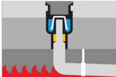
Fire protection insert swells as soon as it comes into contact with fire
