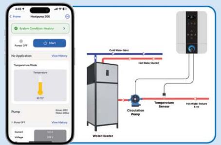
Hot Water Circulation
